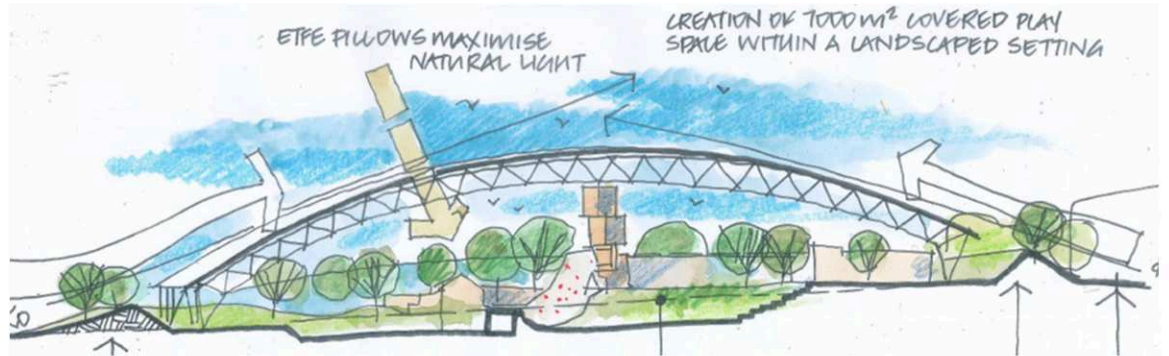
LANDSCAPED BUND CONCEALS SERVICE AREAS, DEFLECTS PREVAILING WIND + VISUALLY CONNECTS SKYDOME TO ITS LANDSCAPE
